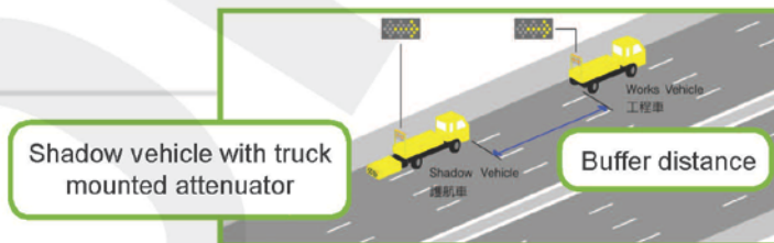
Figure 2: Works vehicle shall be escorted by a shadow vehicle
