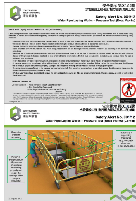
Safety Alert No. 001/12 on Water Pipe Laying Works – Pressure Test (Road Works)
