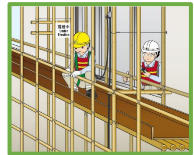
Worker wears a full body safety harness with its lanyard attached to a secure anchorage (e.g. an eye bolt) or an independent lifeline with a fall arrester
