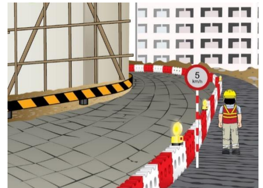
Continuous barriers along access as segregation
