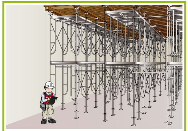
Temporary structure and support inspected by a designated person before use.
