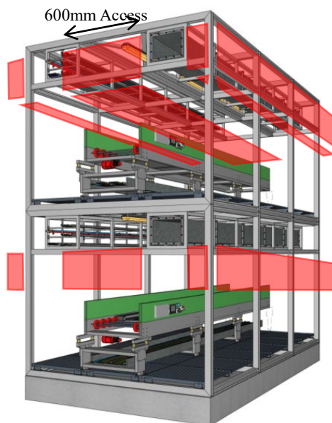
Figure 3.2 Possible configuration of work accesses ('red zones') for horizontal module (Courtesy of AECOM UK)
