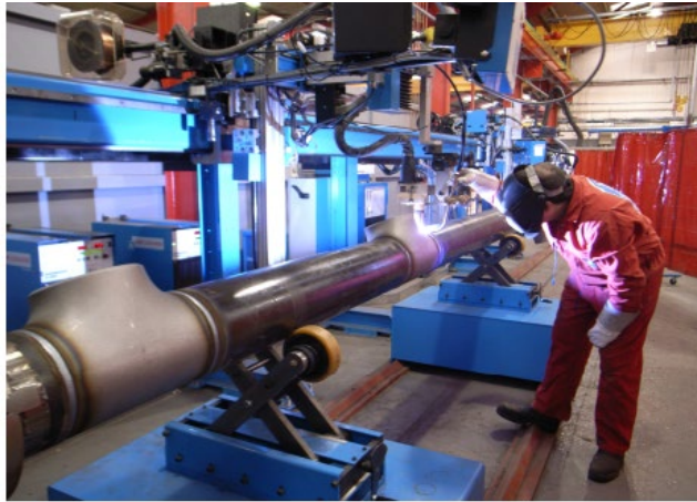
Figure 6.2 Jig for welding pipes (Courtesy of Laing O'Rourke)
