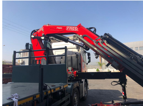
(b) Lifting crane with safe load indicator
