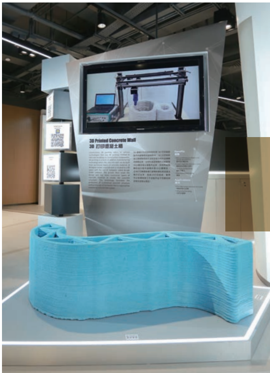
3D Printed Concrete Wall 3D 打印混凝土牆
