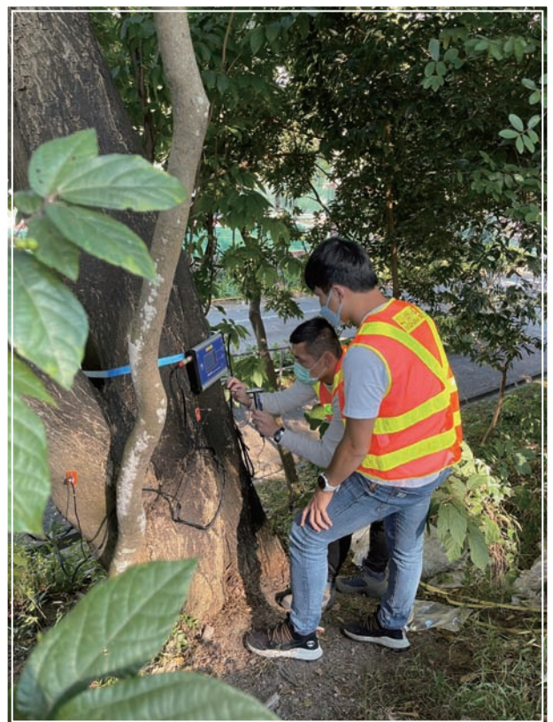
Arborist trainees learn to use sonic tomography to detect trees’ health status
