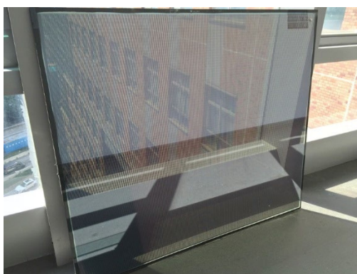
Figure 6 The pictures of vacuum PV glazing
