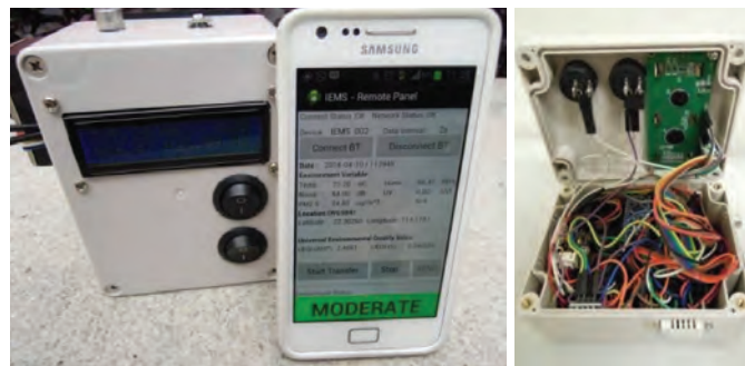
Figure 1 Integrated micro-Environmental Monitoring Device (IEMD) and Android application
