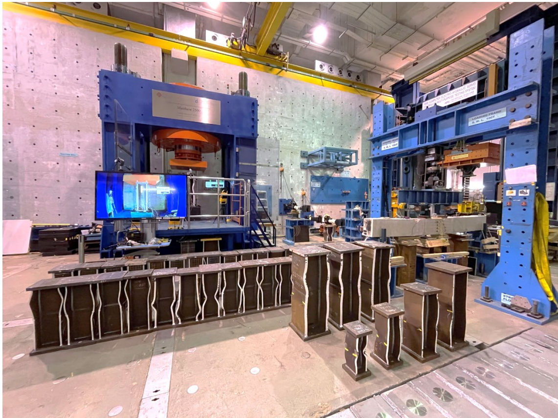
Figure 9.24 Stocky columns and steel piles of S690 welded H-sections with butt-welded splices at mid-height
