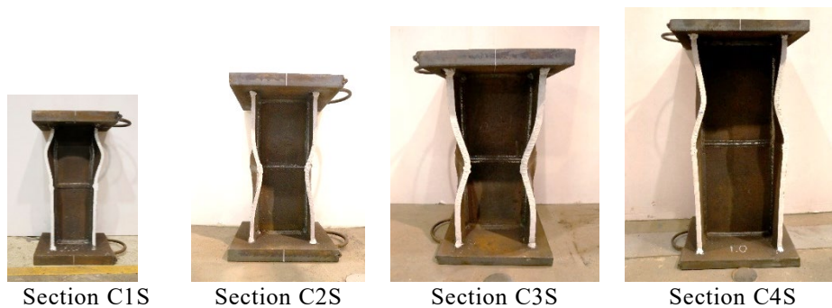
Figure 9.21 Typical failure modes of stocky columns of S690 welded H-sections with splices after testing
