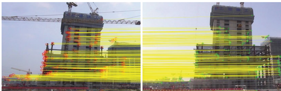
Figure 5 The matching of key points in two images
