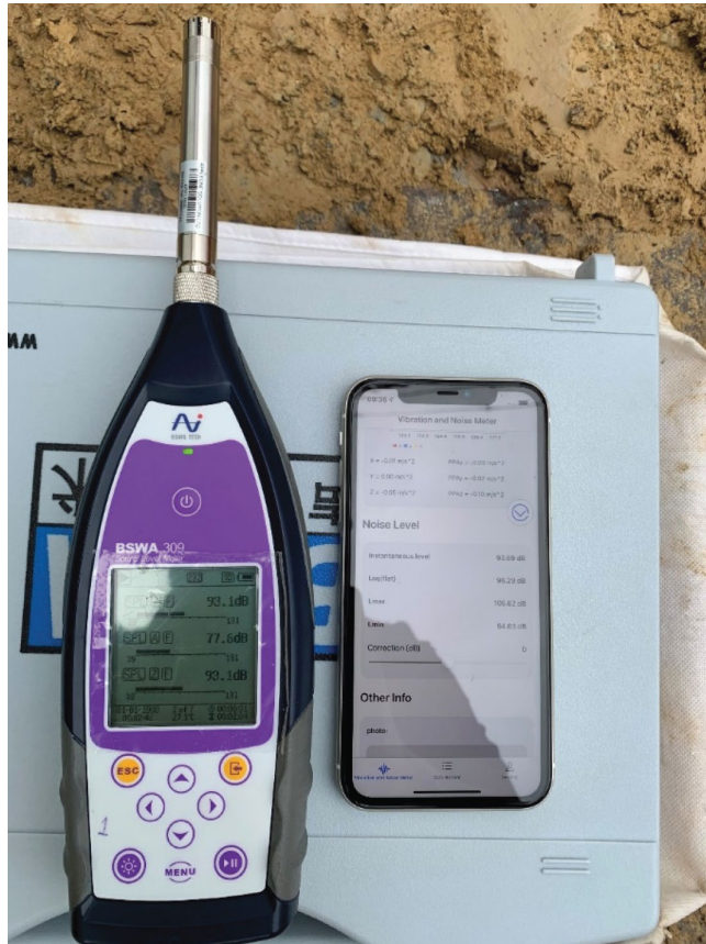
Figure 32 Noise measurement of iPhone 11 and portable sound level meter
