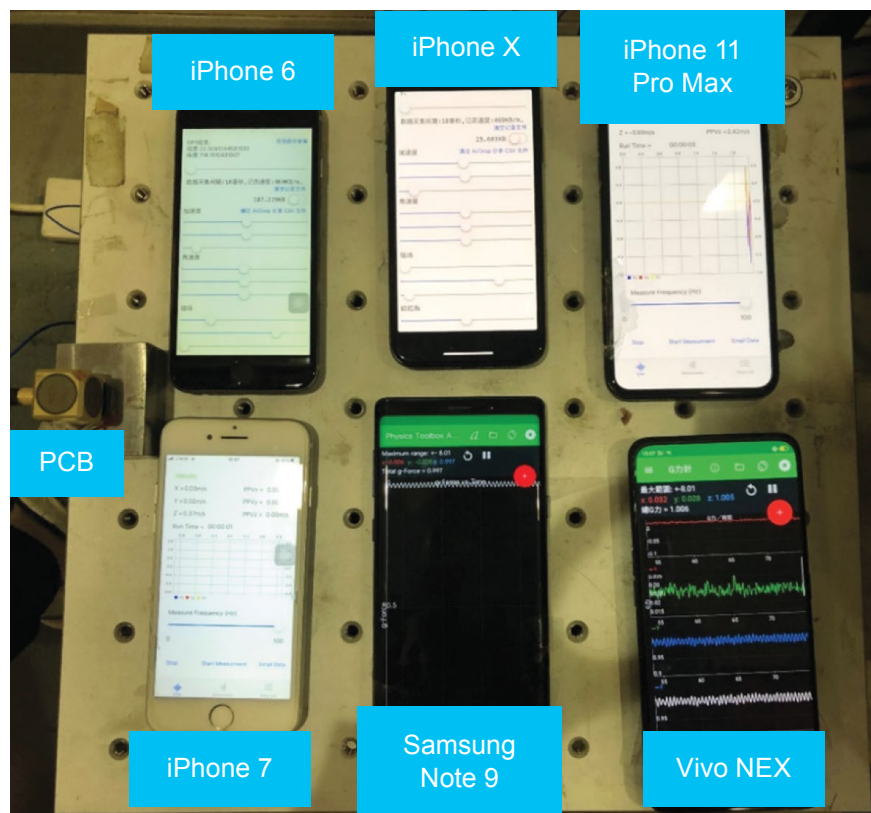
Figure 7 Calibration tests of various smartphone models on a shaking table
