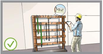
Ensure all lifting gear is provided with valid certificates; clearly marked with its safe working load and an appropriate mark to distinguish it from other similar gear. The lifting gear should also be inspected before use on each occasion.
