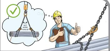
Ensure the safe working load of any multiple sling leg is not exceeded as a result of the angle between the multiple sling legs. Their upper ends shall be connected by means of a
