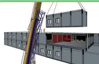
透過使用MIC「組裝合成」建築法將工序由地盤轉到廠房內安裝 Adopting MIC (Modular Integrated Construction) to transfer the operation from site to factory
