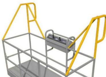
Figure 2: Secondary Guarding Device – Physical Barriers
