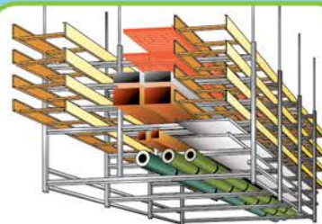
透過使用DfMA (裝配式建築方法) 減少高空工作 Adopting DfMA (Design for Manufacture Assembly) approach to reduce the need for working at height
