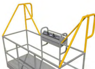
Figure 2: Secondary Guarding Device – Physical Barriers
