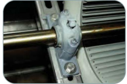
Figure 8 - Sleeve Bearing
