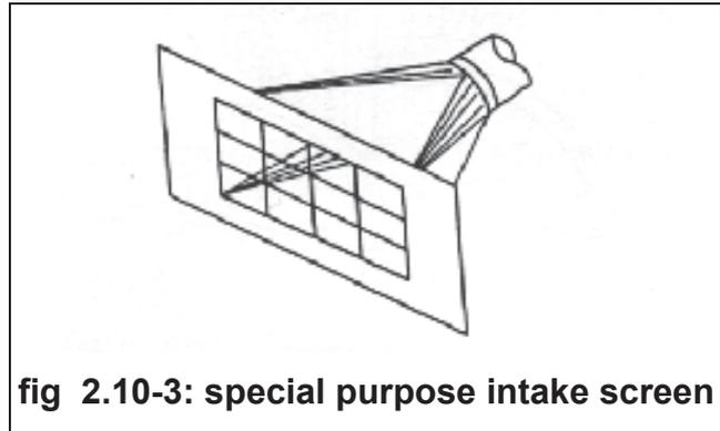
**fig 2.10-3: special purpose intake screen**
