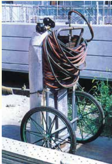
After organization, Gas cylinders stored upright in trolley ready for use
