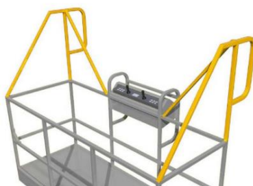
Figure 2: Secondary Guarding Device – Physical Barriers
