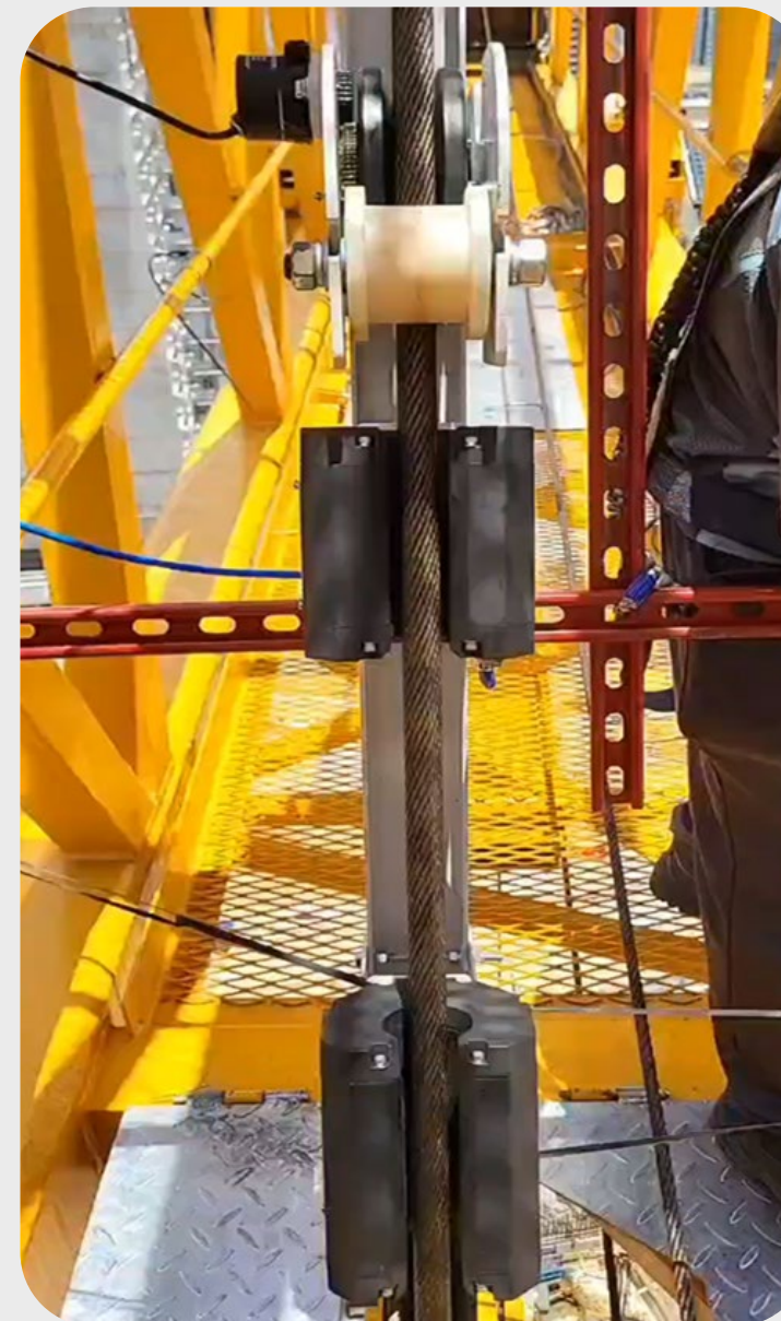
Wire damage presented rapid change in magnetic field
