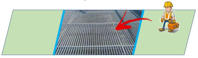
The **ENGINEER** who supervise the construction of this grating deck should make sure that these grating panels are installed properly to avoid accidental displacement.
