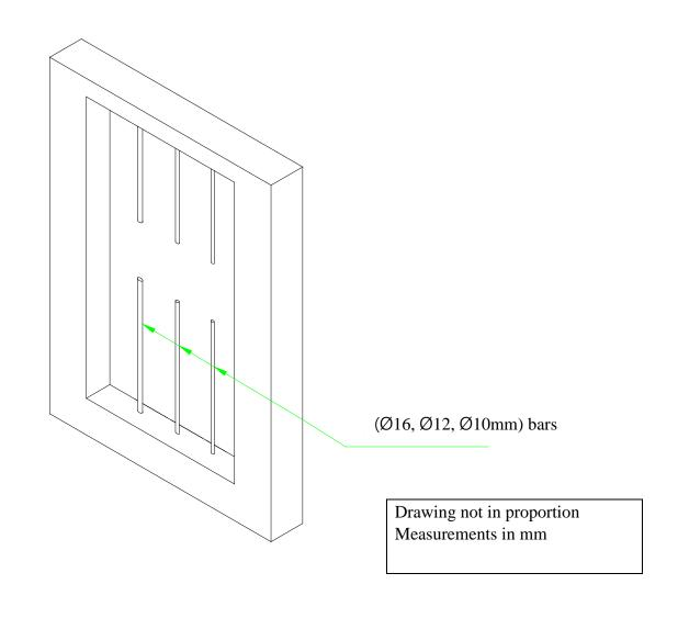
**Bar Joining Test Position**
