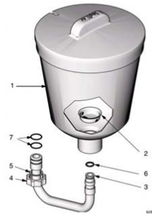
Figure 5-17: Technical details of the Hopper kit as the paint supply vessel
