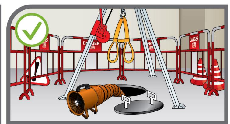
The confined space has to be adequately purged and sufficiently cooled and ventilated before entry of any certified workers and effective measures shall be taken to prevent ingress or in-rush to the confined space of hazardous gas, vapour, dust, fume or free flowing solid or liquid. These measures include blanking off pipelines and service pipes with contents that could cause hazards to health.
