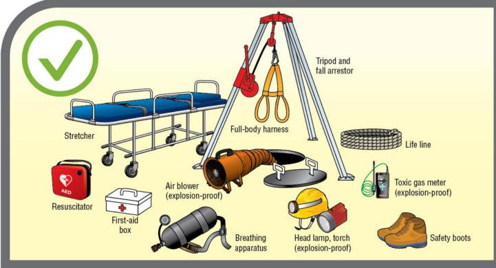
Suitable Personal Protective Equipment and Rescue Equipment shall be provided and maintained for readily use.
