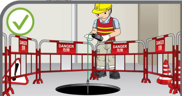
Before entering into the confined space, atmospheric testing shall be carried out to ensure that it is safe for certified workers to enter.
