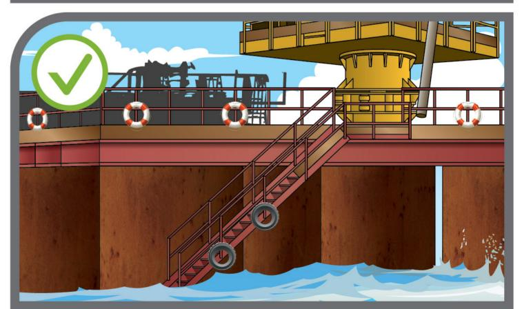
Working platforms over water shall be provided with proper guard-rails, toe-boards, safe access and egress and suitable rescue equipment.
