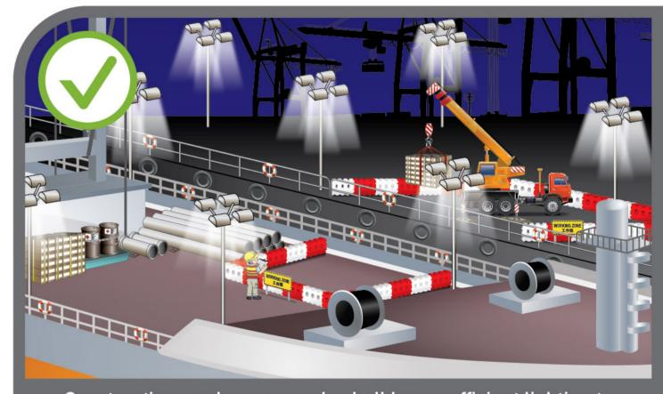
Construction works on vessels shall have sufficient lighting to ensure marine traffic and work safety.
