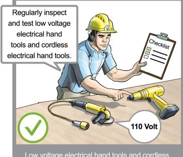
Low voltage electrical hand tools and cordless electrical hand tools should be inspected and tested regularly by a competent person.
