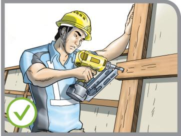
Using cordless electrical hand tools can minimise tripping accidents on site and improve housekeeping and productivity.
