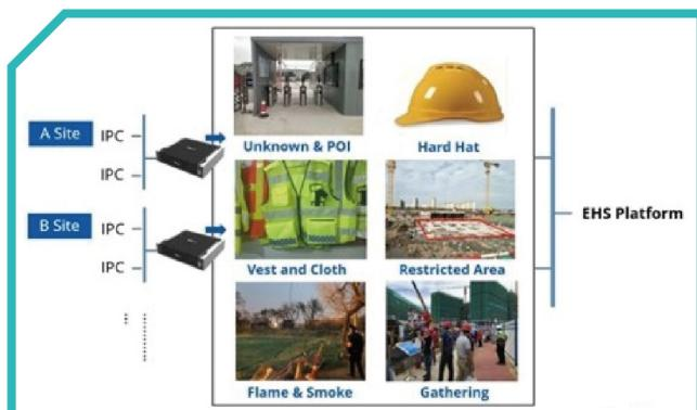
Figure 7 - Safety Monitoring System Using Artificial Intelligence
