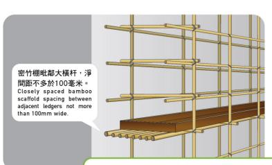
竹棚架每個棚層均應鋪設工作平台。如整個竹棚架為密竹棚 式設計,則須在各棚層每個工作位置架設合適的工作平台。 A working platform should be laid on every lift of a bamboo scaffold. If the entire scaffold is designed as a closely spaced bamboo scaffold, a suitable working platform shall be erected at every working location on a lift.
