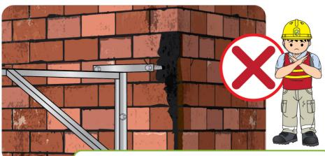
繫穩螺絲的底部結構物料應有足夠的強度和穩定性(例如混 凝土),不應把吊棚錨固在磚牆上或不適當的牆身批盪上。 The base materials of anchor bolts (e.g. concrete) should have adequate
