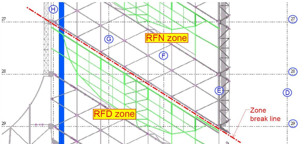
Figure 4 BIM Model Zone Break Line at North - Roof
