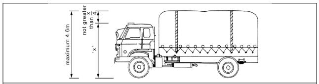
Note: Height of load should not normally extend above the roof of the cab by more than ¼ of the height of the cab from the ground, except in the case of specially designed and enclosed vehicles. Also, the load must not extend beyond the specified overall height of the vehicle (i.e. 4.6 m for medium/heavy goods vehicle or 3.5 m for light goods vehicle).
