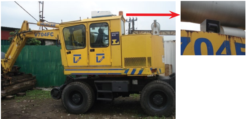
Figure 4 – Camera setup for excavator
