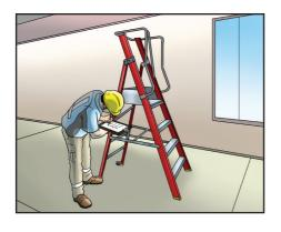
Before use, inspection (including visual check) of the light-duty working platforms according to the safety checklist provided by the supplier or other equivalent safety checklist should be conducted.
