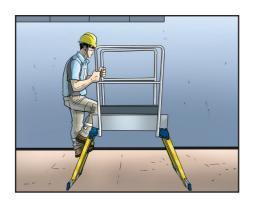
Worker should face the light-duty working platform when ascending or descending.
