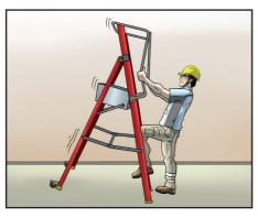
Do not apply excessive force to the working platform and induce lateral force rendering the overturning of the working platform.
