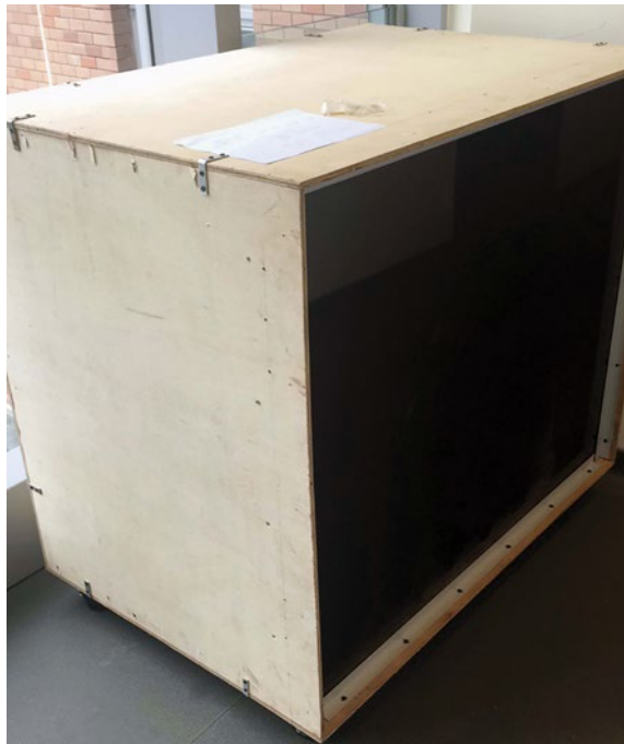
Figure 9 The test chamber mounted with the vacuum PV glazing on the front side
