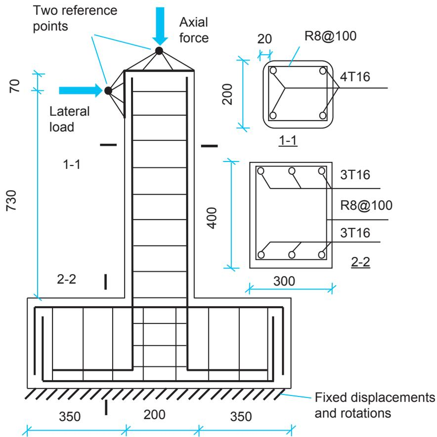
Figure 3 Specimen details (unit: mm)
