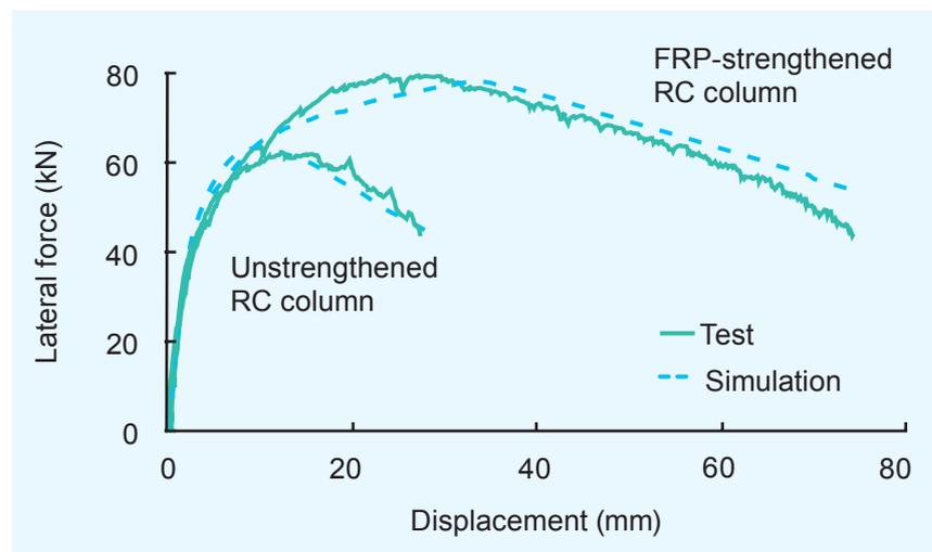
Figure 6 Calibration of the FEM model
