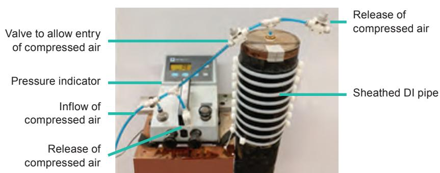
Figure 6 Experimental setup for the pressure test.
