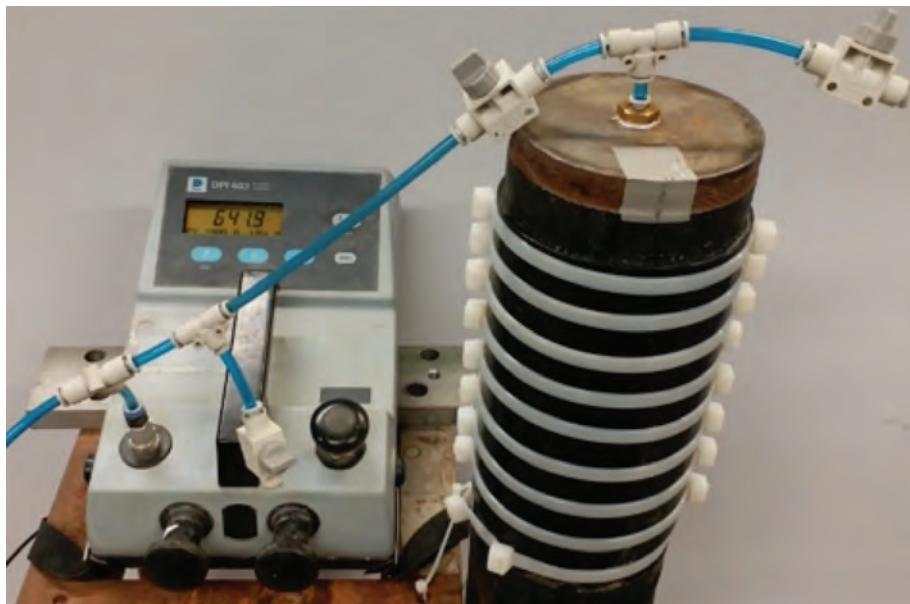
Figure 21 A sheathed DI pipe sustaining a leakage pressure of 640 kPa.
