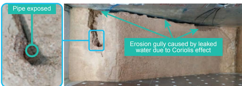
Figure 15 Top view of the slope at the end of Test 7.
