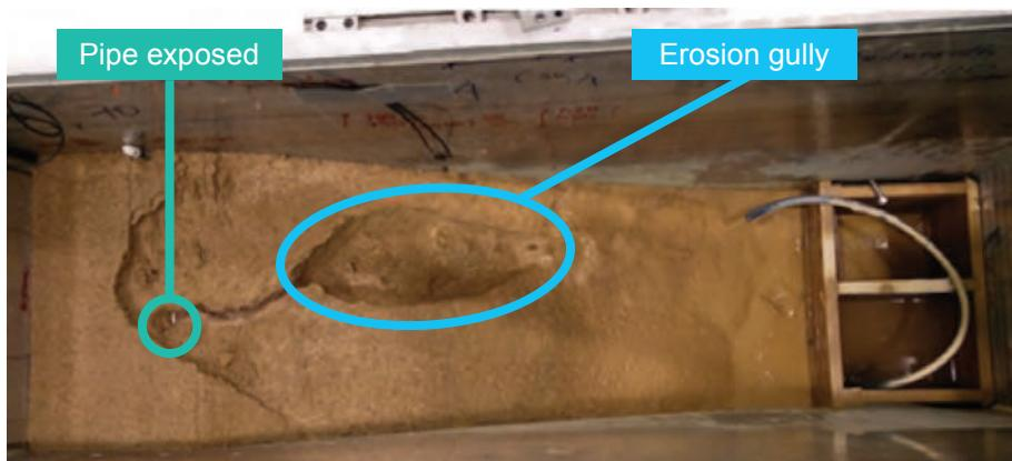
Figure 13 Top view of the slope at the end of Test 1
