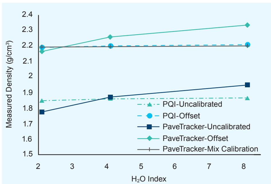
Figure 11 Relationship between H<sub>2</sub>O Index and Measured Density
