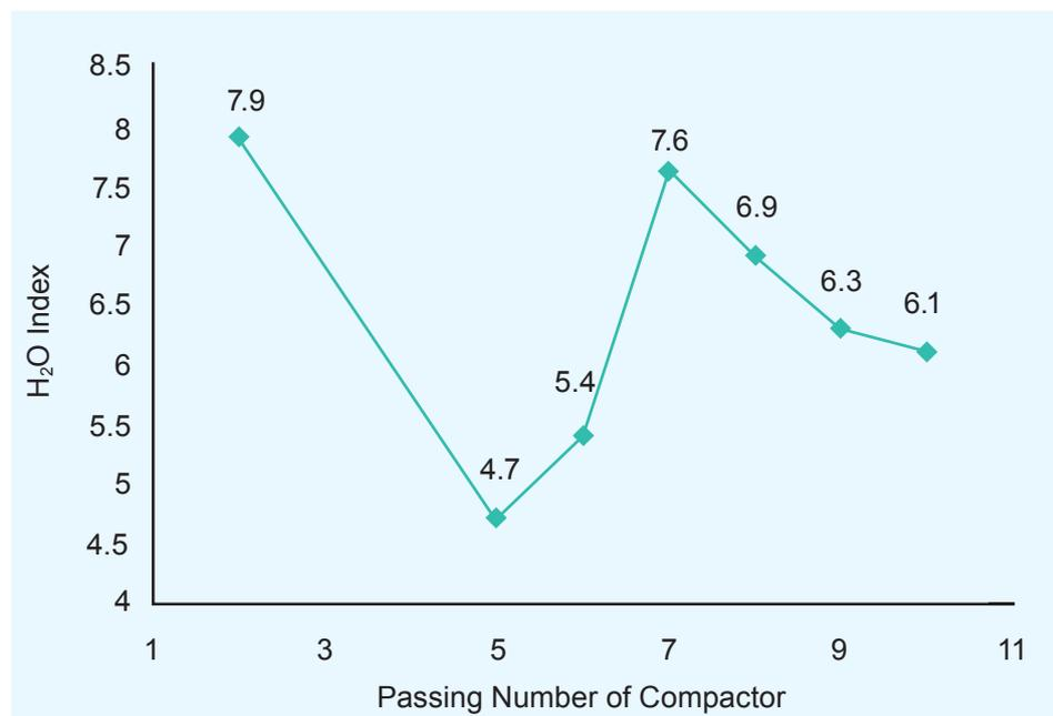
Figure 10 Relationship between Passing Number of Compactor and H<sub>2</sub>O Index
