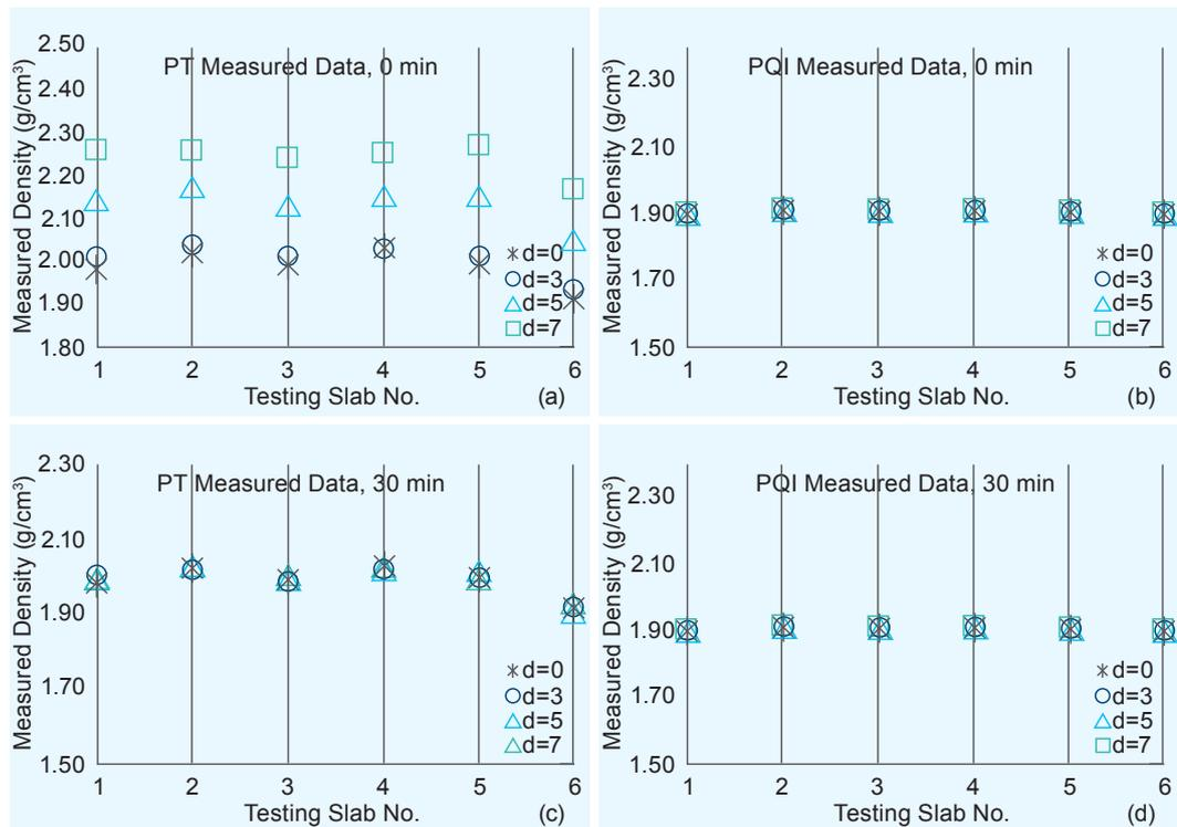
Figure 13 Effect of Painting Area and Volatilization Time on EM Density Gauge Data
