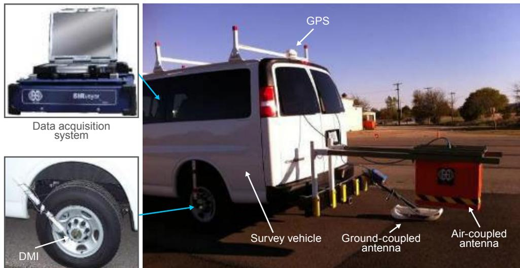
Figure 2 Ground Penetration Radar Measurement System
