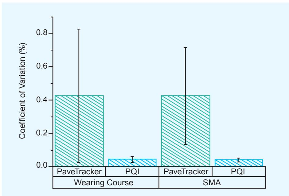
Figure 16 Coefficient of Variation of the EM Density Gauge Data
