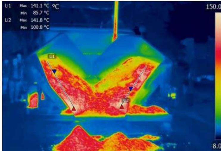
Figure 29 Temperature Monitoring Before Paving
