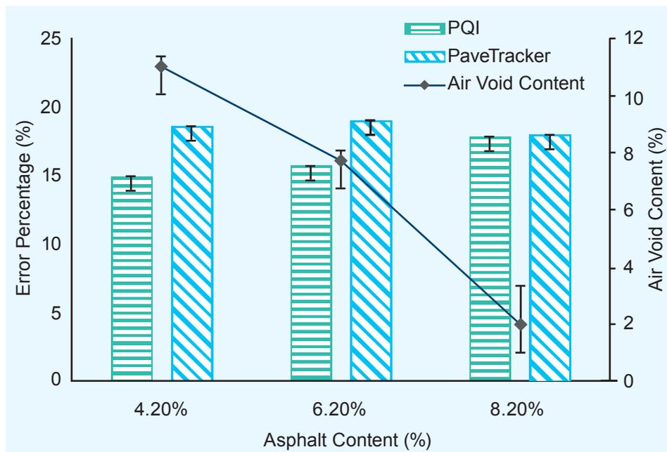
Figure 9 Relationship between Error Percentage, Air Void Content and Binder Content
