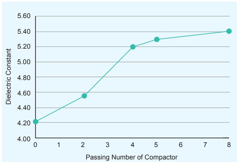
Figure 22 Dielectric Constant versus Passing Number of Compactor (Lau Shui Heung Rd)
