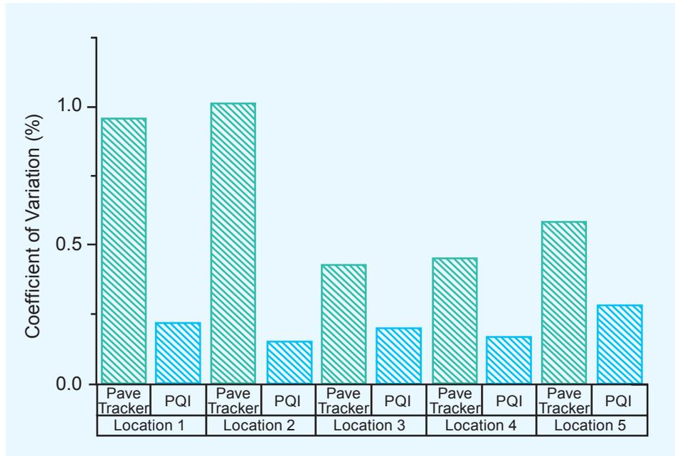
Figure 25 Coefficient of Variation of EM Density Gauge Data at Different Locations
