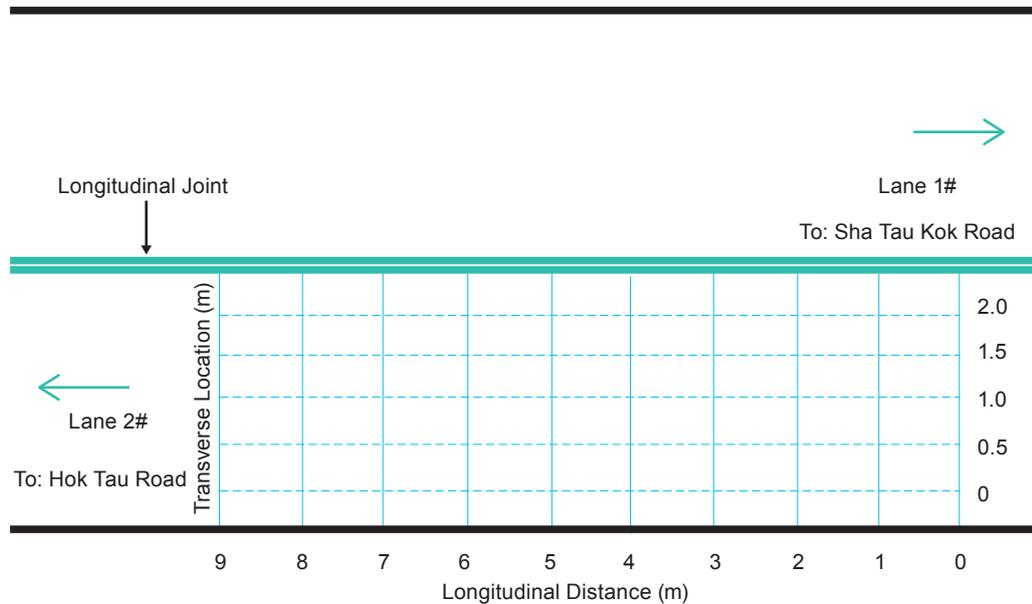
Figure 26 Testing Area Schematic at Lau Shui Heung Road
