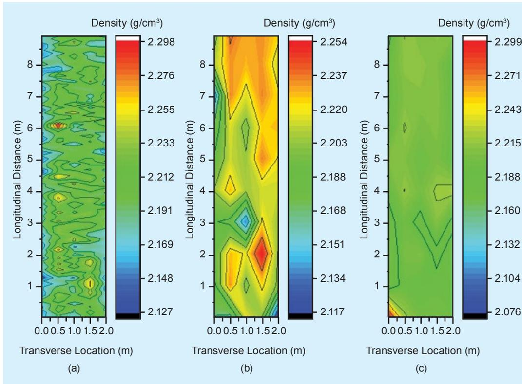
Figure 27 Density Map of Lau Shui Heung Road: (a) GPR, (b) PaveTracker, and (c) PQI
