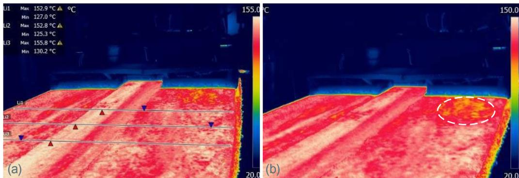
Figure 33(a) & (b) Thermal Image of the Asphalt Pavement during Paving
