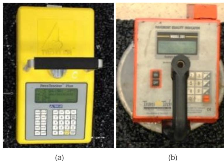
Figure 1 EM Density Gauge: (a) PaveTracker™ Model 2701-B Plus; (b) PQI™ Model 301
