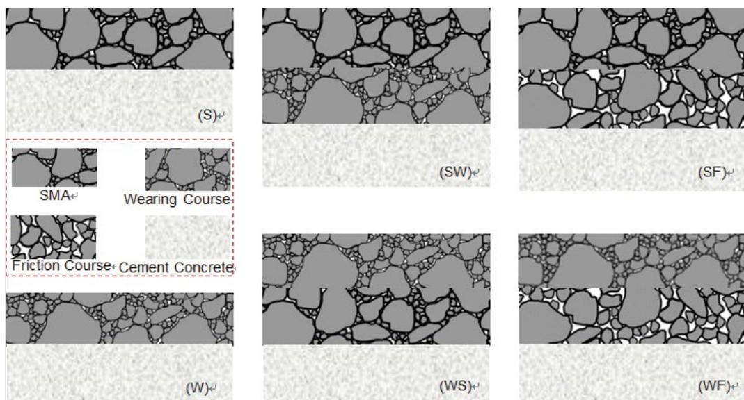
Figure 14 Description of Different Structures
