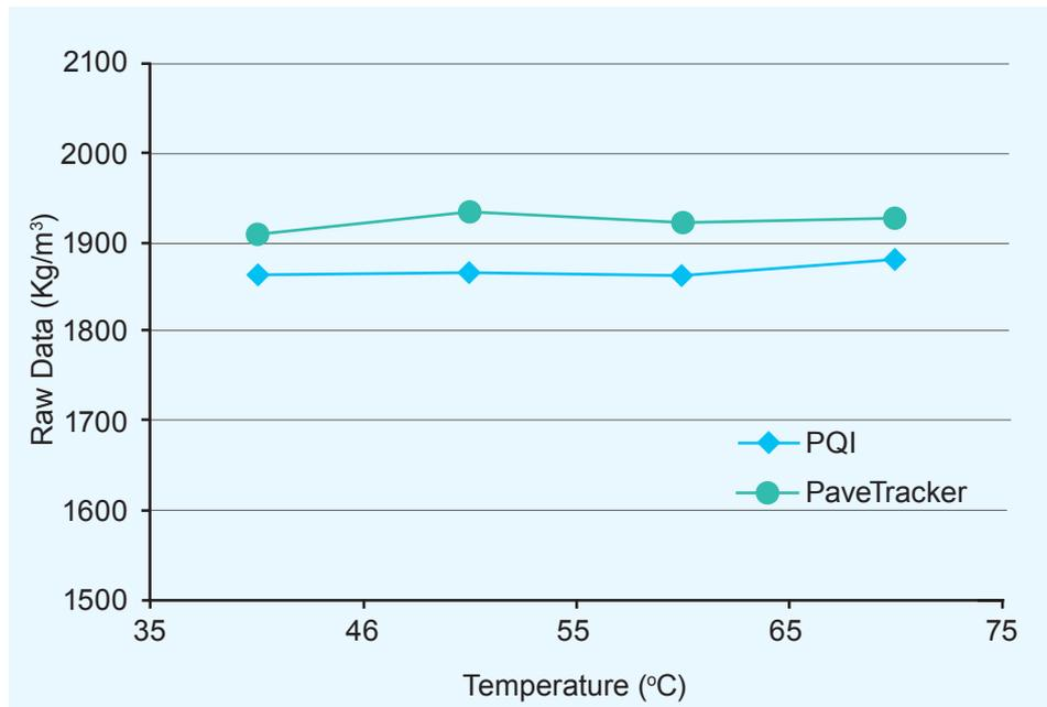
Figure 24 Relationship between the EM Density Gauge Data and Temperature
