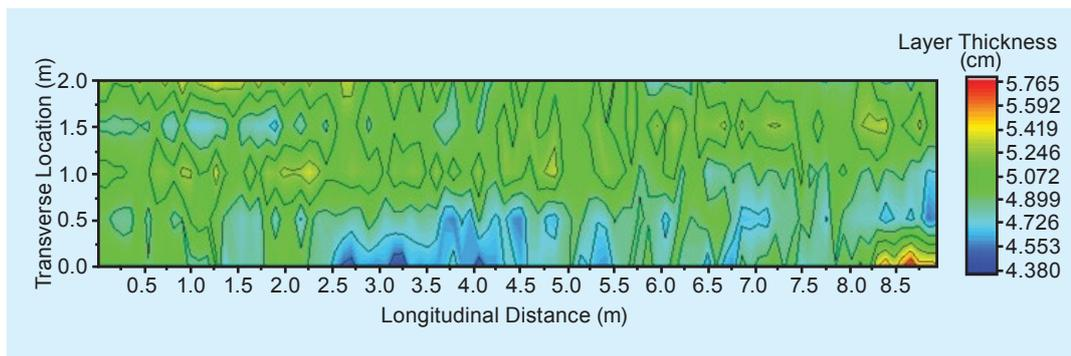
Figure 28 Layer Thickness Map of the Testing Area at Lau Shui Heung Road
