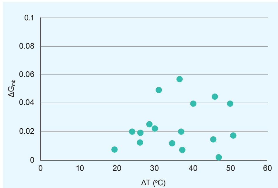
Figure 35 Relationship between Changes in Temperature and Changes in Density
