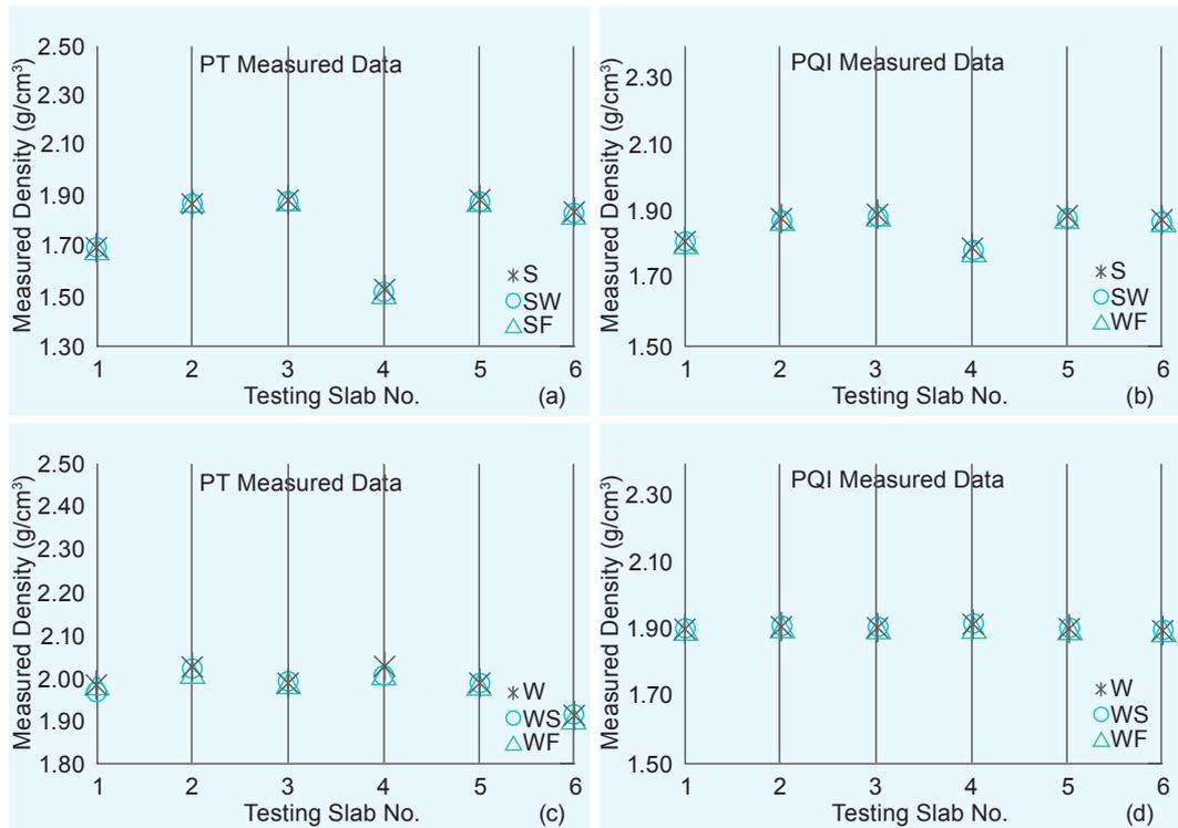
Figure 15 Effect of Underlying Layer on EM Density Gauge Data: (a) PT collected raw data from S, SW, and SF, (b) PQI collected raw data from S, SW, and SF, (c) PT collected raw data from W, WS, and WF, and (d) PQI collected raw data from W, WS, and WF
