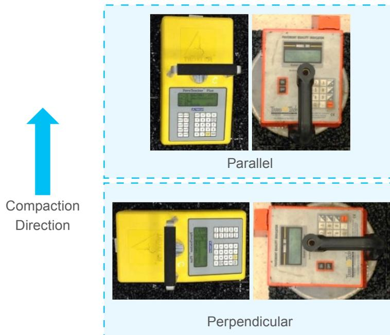
Figure 6 Measurement Directions
