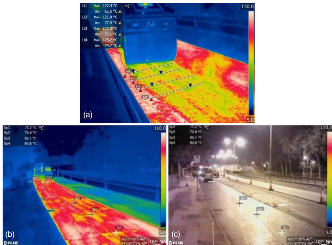
Figure 31 Temperature Monitoring During Compaction
