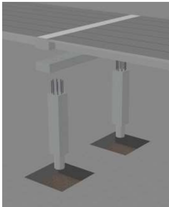
Figure 6.4 Exploded view of HfL precast bent concept (FHWA, 2013a)
