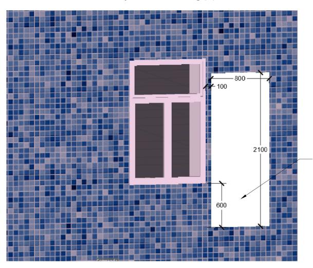
Angle bracket NOT to be installed in this area
