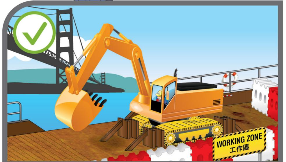
Excavator and other lifting appliances on vessel shall be secured to a fixed location.
