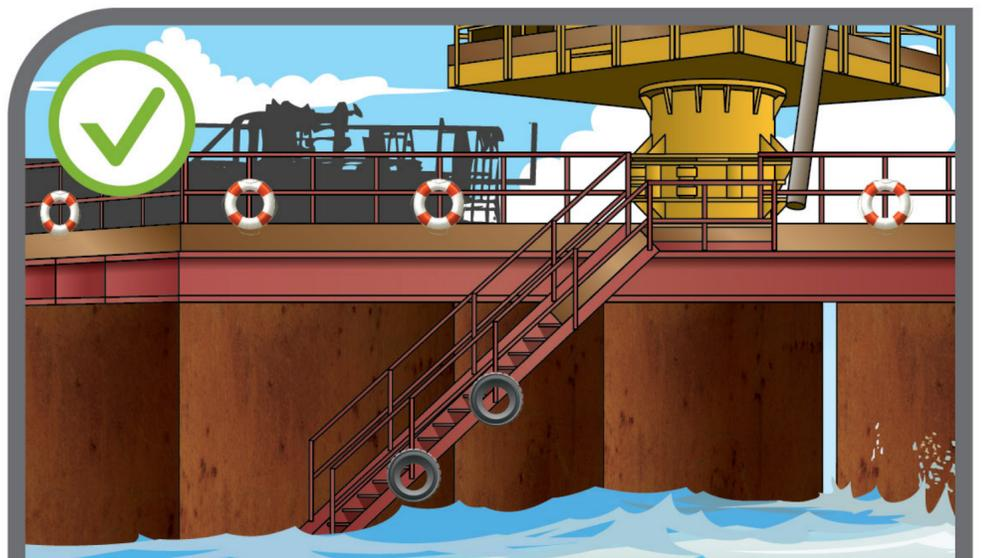
Working platforms over water shall be provided with proper guard-rails, toe-boards, safe access and egress and suitable rescue equipment.
