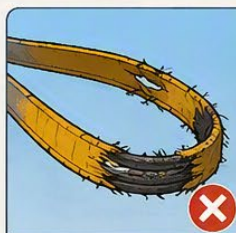
吊具/索具損壞
