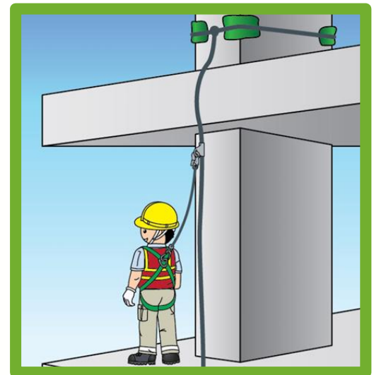
When dismantling working platform, a worker must wear a full body safety harness with its lanyard attached to a secure anchor point or an independent lifeline with a fall arrester
