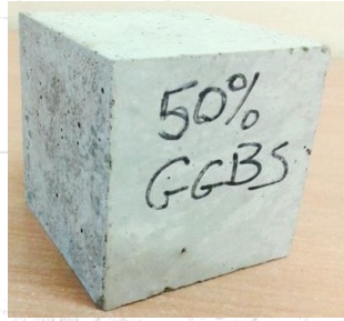
High cement replacement concrete in structural element without rapid strength development required
