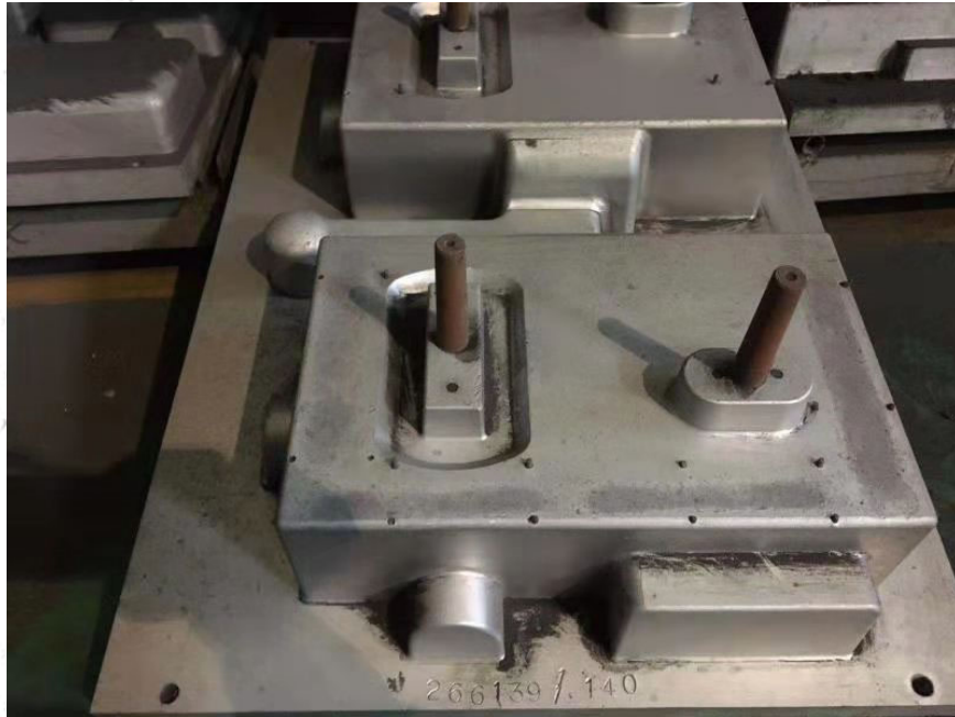
Die Cast Mould of Connection Box Reuse for 20,000 times
