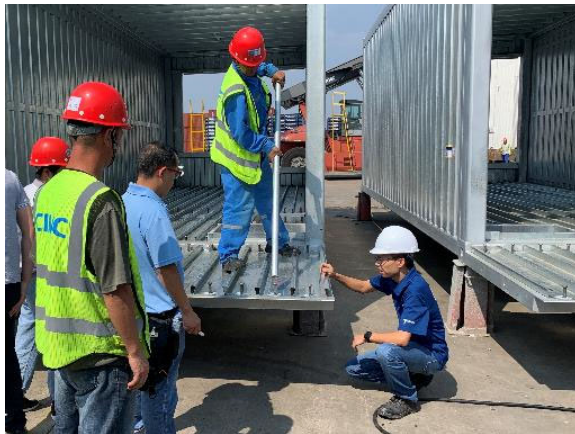
Bending test of shear stud
