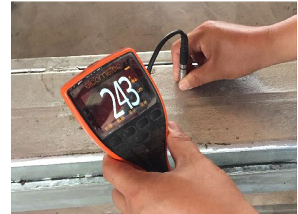
Measurement of thickness of galvanizing layer
