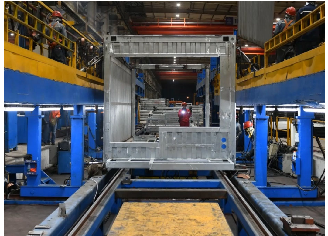
6. Module assembly (~0.5 days)
