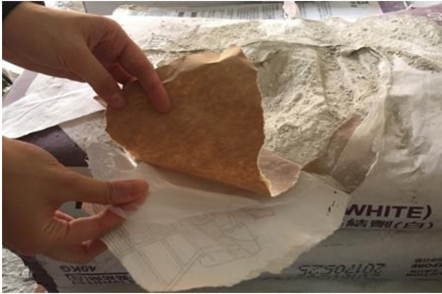
Photo 25: 3-Layers Packaging for Tiling Agent (Kraft Paper, Plastic Wrap and Paper)
