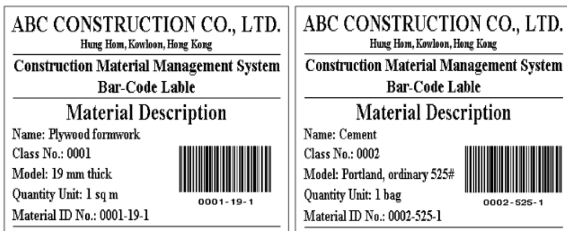
Figure 7 Sample bar-codes for construction materials (Chen et al., 2002)
