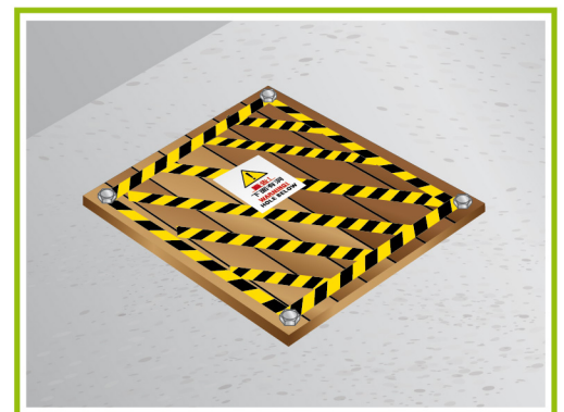
Use of secured covering with warning notice.
