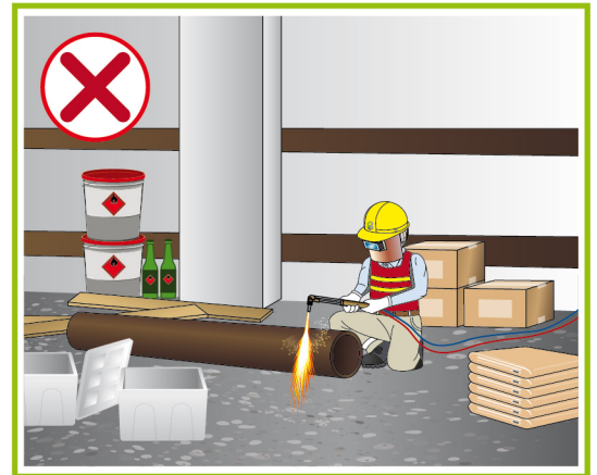
Do not conduct gas welding and flame cutting operation adjacent to the flammable substances.
