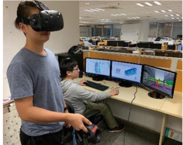
Figure 1.2 Use of virtual reality to rehearse the installation of MEP works (Courtesy of FSE Engineering Group Ltd.)
