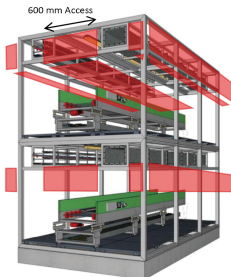
Figure 2.9 Possible configuration of work accesses for horizontal module (Courtesy of AECOM UK)
