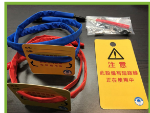
Figure 2 (8.1.1c.iii): Temporary Jumper
