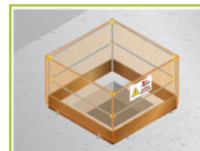
Provide guard-rails, toe-boards and warning signs at the floor opening.
