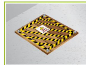
Use of secured covering with warning notice.
